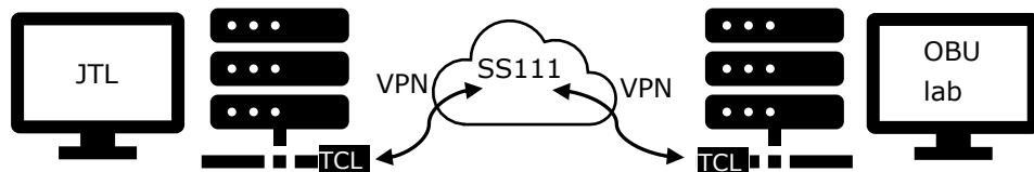
Figure 2: Connection facilities for remote JTL testing
